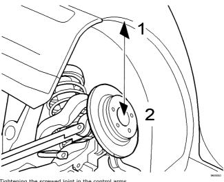
Tightening the screwed joint in the control arms
